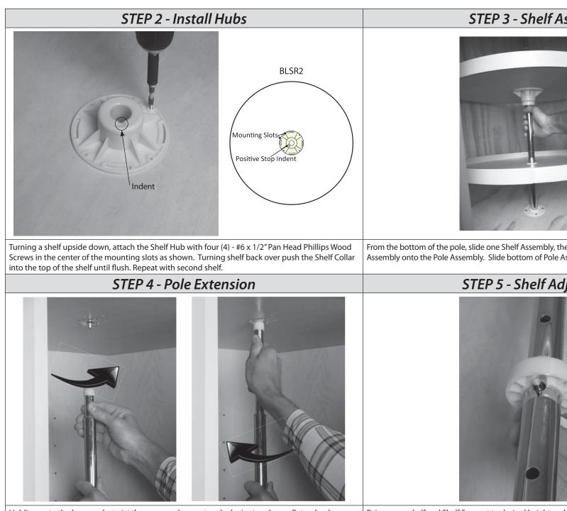
Holding onto the lower pole, twist the upper pole counter-clockwise to release. Extend pole upwards until it rests firmly against the Top Mounting Bracket and tighten by turning the upper pole clockwise.
